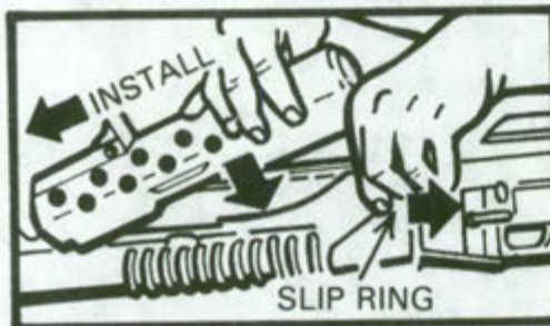
c. INSTALL HANDGUARD AND SECURE WITH SLIP RING.
