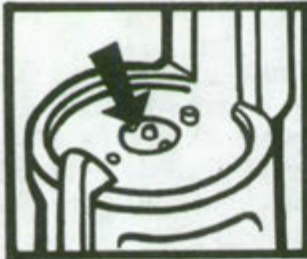
CHECK FOR LOOSE BREECH INSERT.
