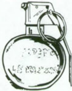
Figure 1. M33, FRAGMENTATION HAND GRENADE. Color/Markings - OD with single yellow band and printing.
