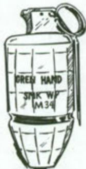
Figure 3. M34, WP SMOKE HAND GRENADE (STANDARD COLOR AND MARKINGS). Color/Markings - Light green, yellow band, red printing. Old Markings - Light gray, yellow band, yellow printing.
