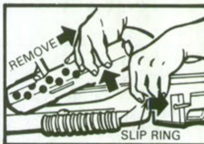
PULL BACK SLIP RING. LIFT UP ON HANDGUARD AND PULL TO REAR TO REMOVE.
