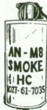
Figure 4. AN-M8, HC SMOKE HAND GRENADE. Color/Markings - Light green, black printing, white top. NOTE: M18 Colored Smoke looks the same but the top is the same color as the smoke.
