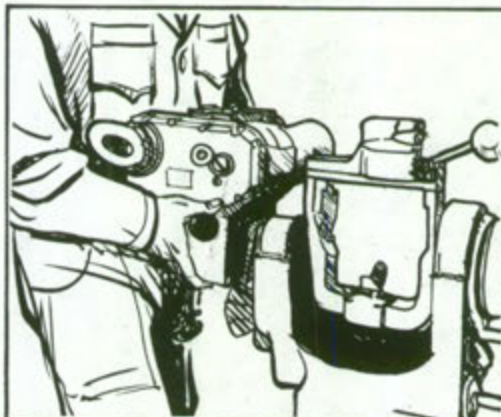
Figure 9. Alinement of sight and boresight plate.
