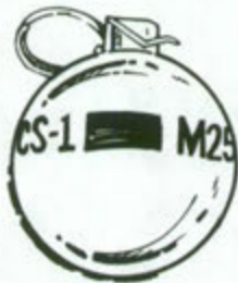
Figure 2. ABC-M25A2, CS RIOT CONTROL HAND GRENADE. Color/Markings - Gray, red band(s) and red printing.
