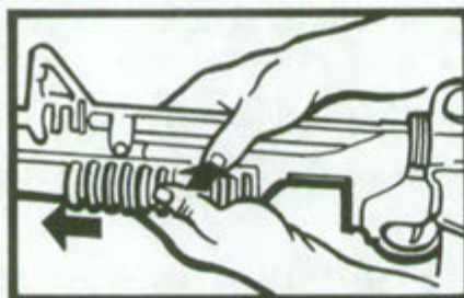
c. PRESS BARREL LATCH AND MOVE BARREL FORWARD TO STOP.
